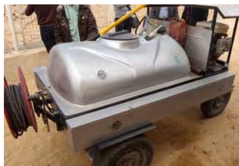
Photo 2-2-14 PV washing machine using high pressure water
