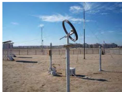
Photo 3-1-3-2 Pyranometers set in Hurghada meteorological observatory
