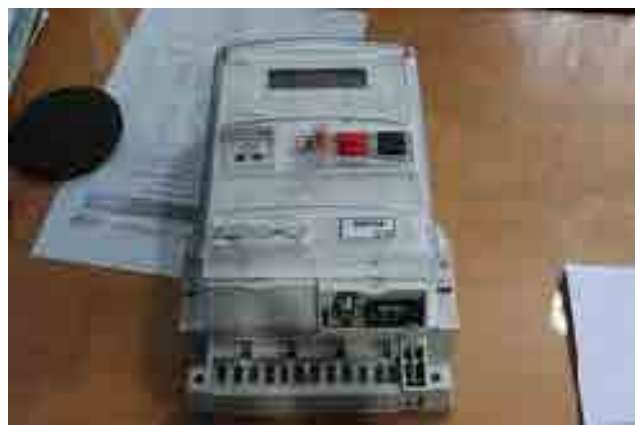
Typical Energy Meter with Remote Reading Facility
