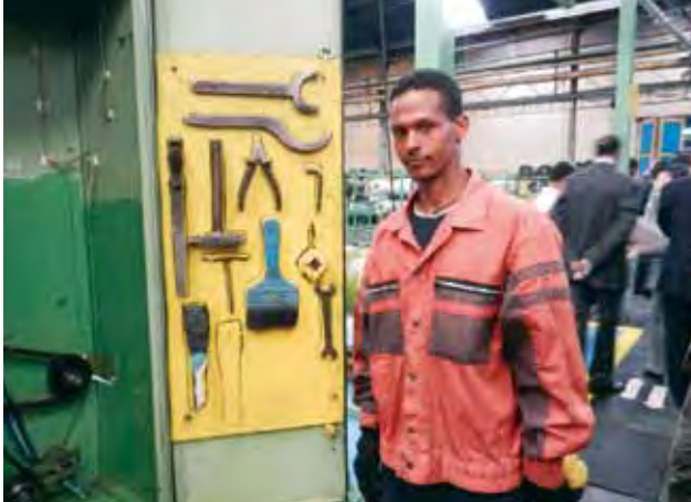
The 5S program was introduced at this Ethiopian factory participating in the KAIZEN project.
