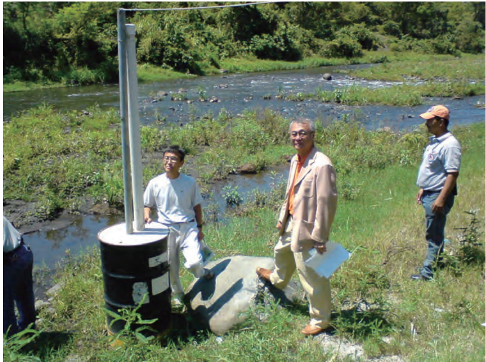
Figure 9: Water Glass (Water Level Monitor) with Automatic Warning System in Guatemala
