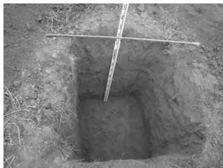
GL to 1.15m: Topsoil with weathered hard laterite. Deeper than 1.15m: Manual excavation is possible but hard due to rather hard laterite. Long-term allowable bearing capacity: Over 5t/m 2
