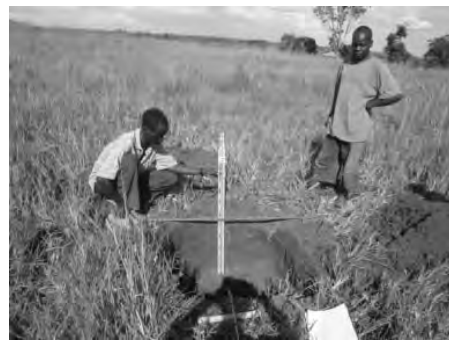
GL to 0.73m: Top soil of medium sandy clay. Deeper than 0.73m: Difficult to excavate manually due to hard laterite. Long-term allowable bearing capacity: Over 10t/m 2 .
