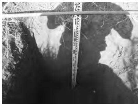
GL to 1.12m: Top soil of medium sandy clay. Deeper than 1.12m: Difficult to excavate manually due to hard laterite. Long-term allowable bearing capacity: Over 10t/m 2 .
