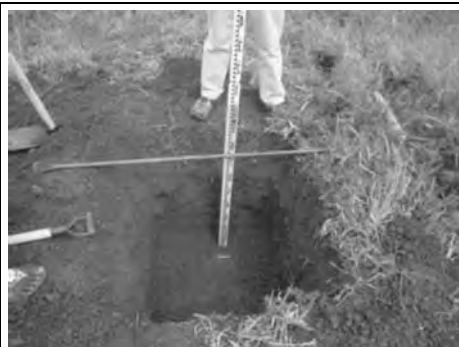
GL to 0.70m: Top soil of clay with small particle of laterite. Deeper than 0.70m: Difficult to excavate manually due to hard laterite. Long-term allowable bearing capacity: Over 10t/m 2
