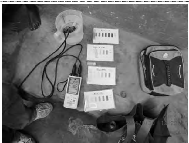
Rapid water quality test - Temperature 26.0°C, pH 6.33, EC 21.8mS/m, F 0mg/L, HNO 3 0mg/L, HNO 2 0.02mg/L, Fe 0.3mg/L - suitable for drinking. (Unyama RGC)
