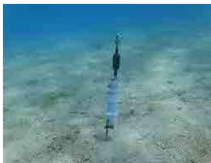
Fig. 5.2.2-2 (3) Current meter at St.C2
