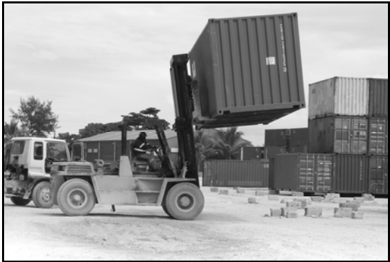
Photo 1.2-6 Handling by Forklift
