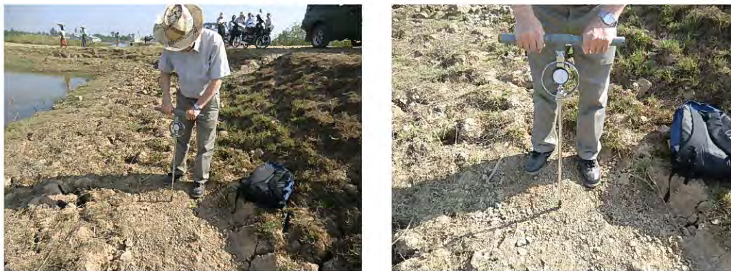
Photo-2-2-1 Cone penetrometer test
