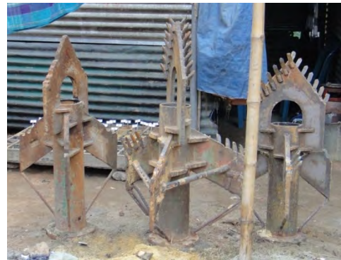
Figure 2.2.2 Blade Bits for Drilling of Sand, Gravel and Clay Layers (Made in Bangladesh)
