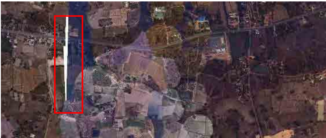
Figure 2.2.69 Example of Broken Sidelap
