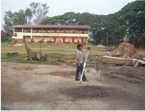
Figure 2.2.6 Implementation of Ground GPS Observation (March 20, GCP-03)
