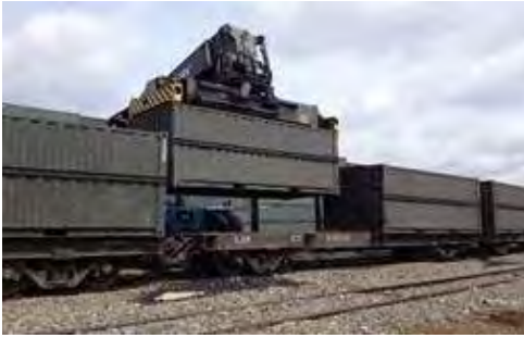
Unloading container from wagon
