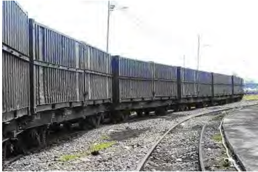
[Pic. 4-5-2] PPCW Type Container Wagon
