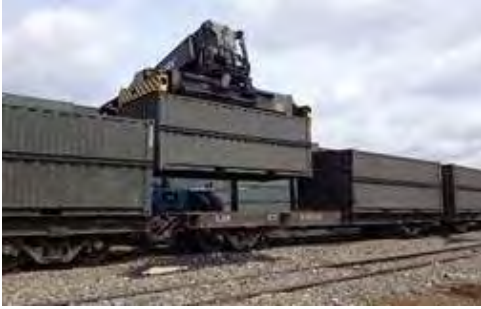
Unloading container from wagon
