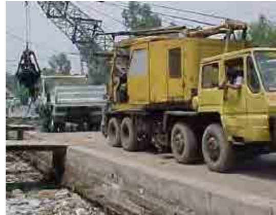
Presently Owned Bucket Crane (Mechanical Rope Type Clam Shell)
