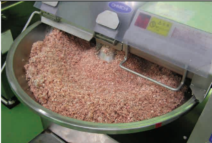
Cutting of semi-frozen lean pork and pork back fat with starter culture Temperature of mixture; -7 to -5°C,
