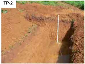
$k = k = n \times 10^{-3}$  cm/sec. In addition, it is expected that the high ground water table confirmed in this test pit would function as a barrier against the seepage passing through the abutment.
