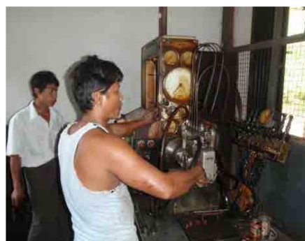
Adjusting Work of Fuel Nozzle of a Engine [AMD Medium WorkshopNo.4]
