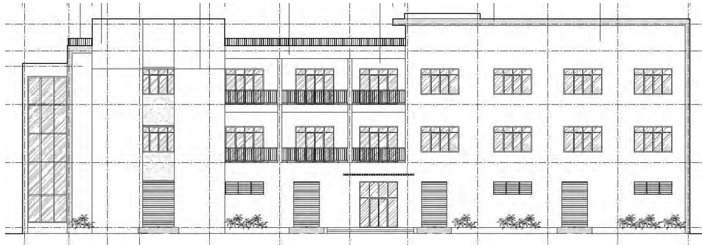
Figure 3.5.12 South Face of Administrative Building Elevation Plan
