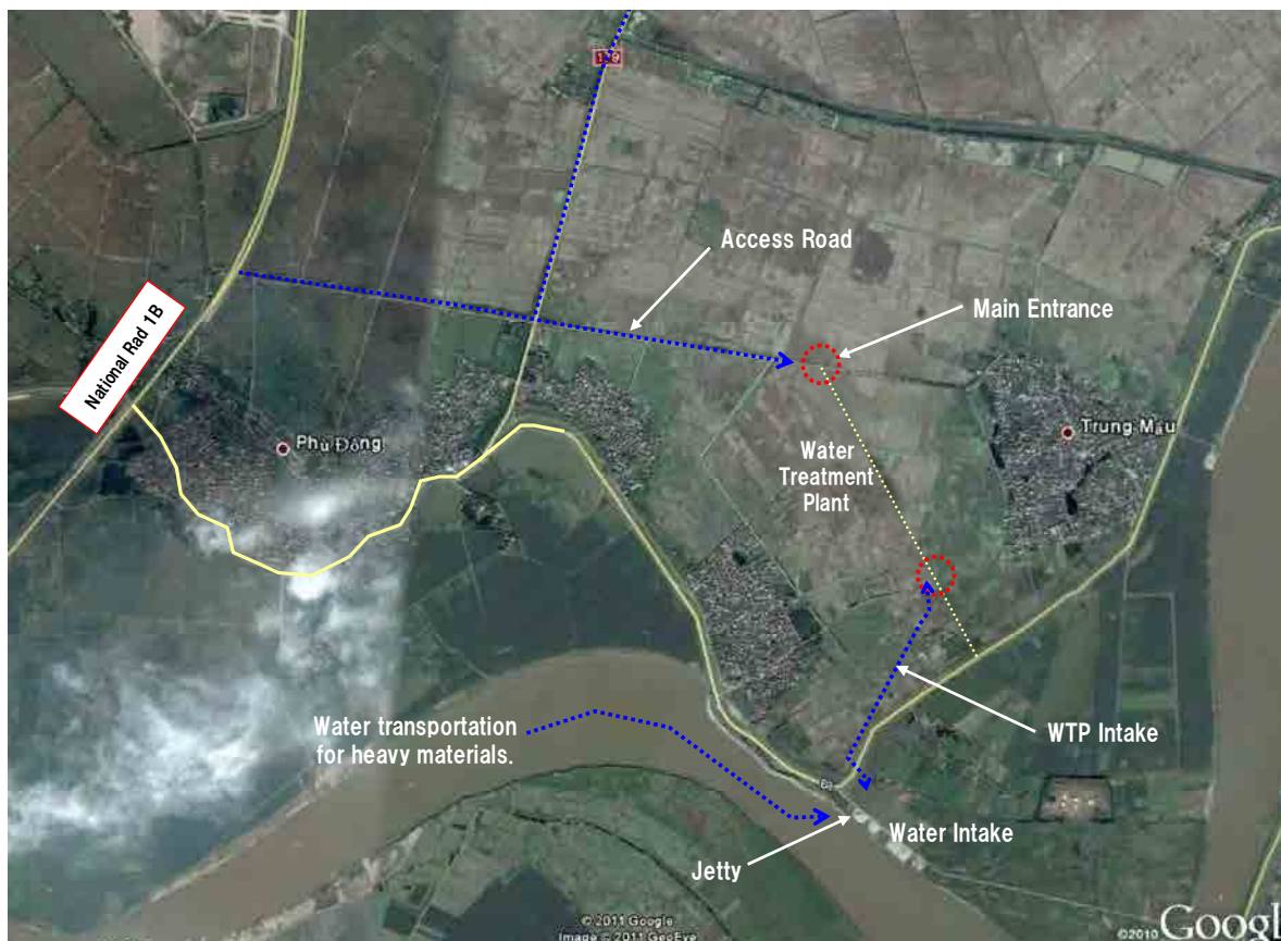
Figure S.24 Approach Roads for Construction
