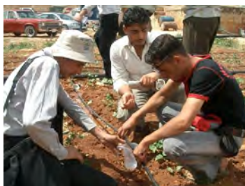
A scene of measuring discharge by the "discharge measurement kit"
