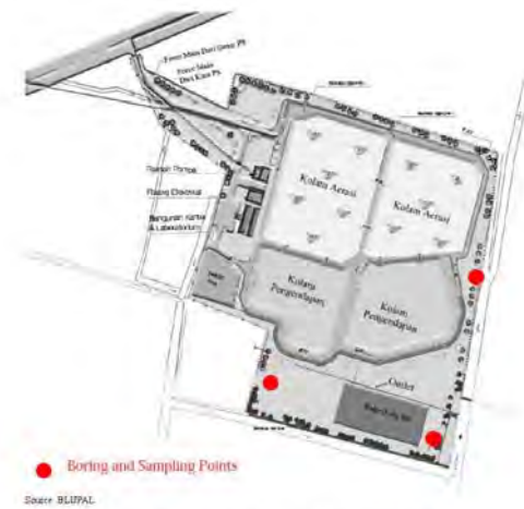
Figure 1 Boring and Sampling Locations at the Suwung WWTP
