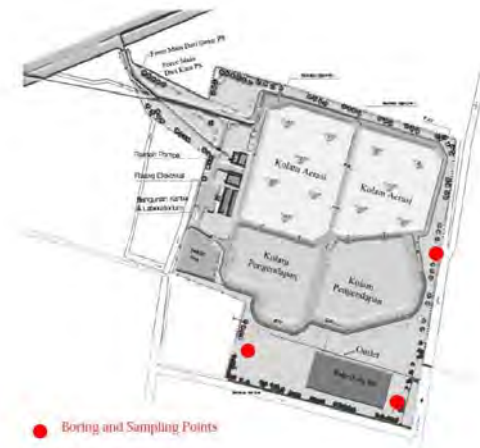
Figure 1 Boring and Sampling Locations at the Suwang WWTP
