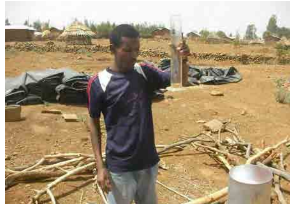
A DA measures rain fall amount by using measuring cylinder in FTC, Bugena Woreda
