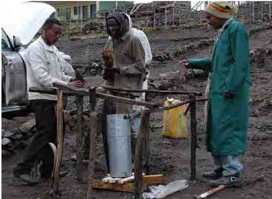
Rain gauge installation in FTC compound in Gidan Woreda
