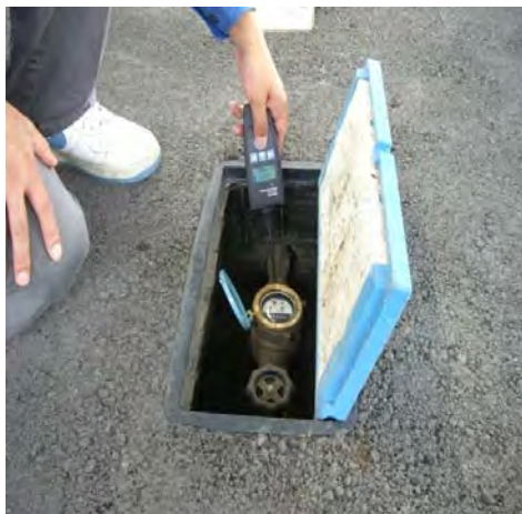
Figure II-2.19 TS Leak Checker: Time Integral Type Leak Detector
