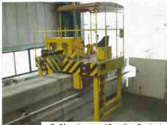
C. Shunting car (Gasoline Engine)
