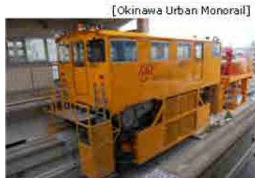
F. Mobile work-shop(coupled with crane car)
