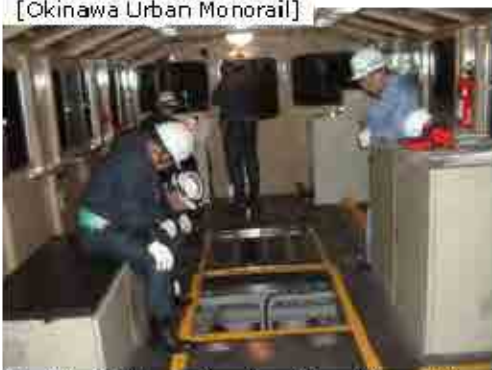
G. Inside Mobile work-shop(Visual inspection of track )
