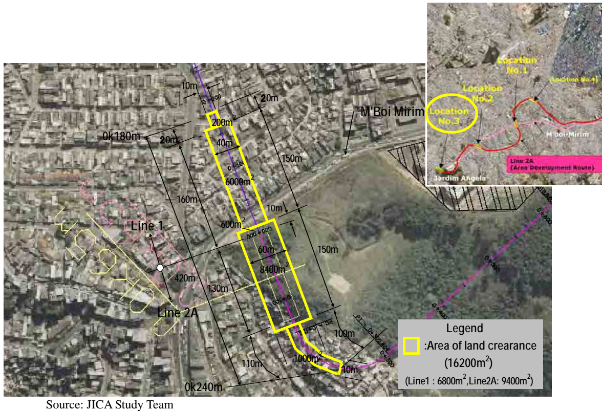
Figure 5-52 Area of land clearance of location No.3
