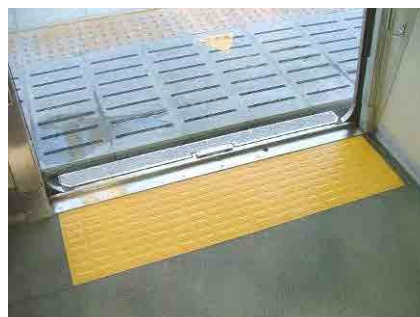
Figure 5-11 Smooth transition of the train and platform
