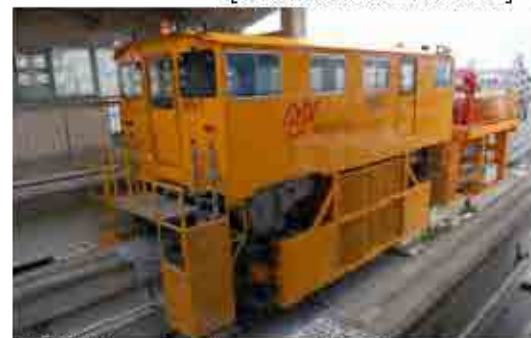
F. Mobile work-shop (coupled with crane car)
