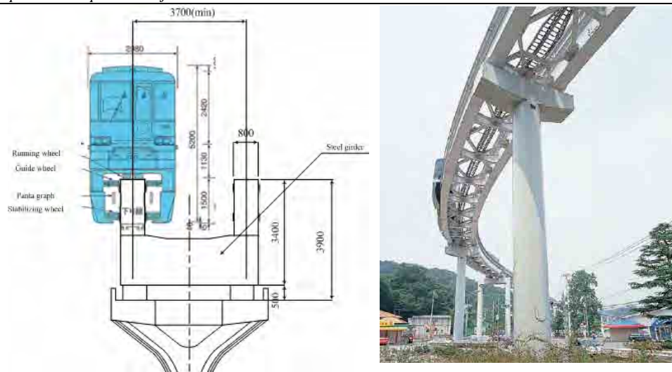
Figure 6-2 Typical Section Drawing and Photo of Steel Girder
