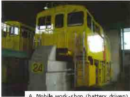
A. Mobile work-shop (battery driven)
