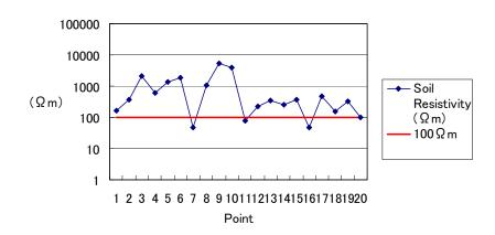
Figure 4.2.10 Measurement of Soil resistivity (Graph)
