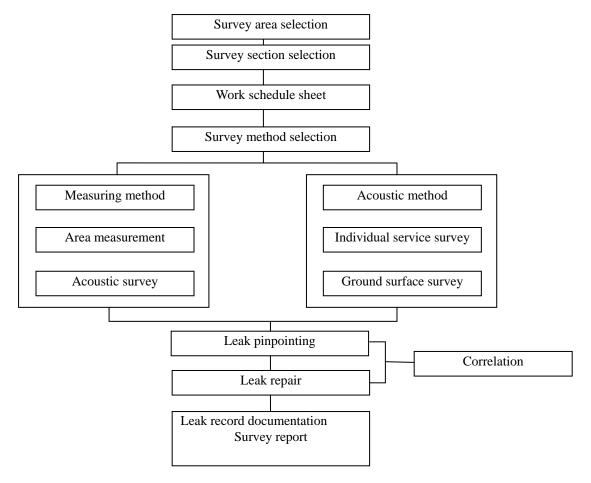
Figure A.3.1 Basic Leak Surveying Flow
