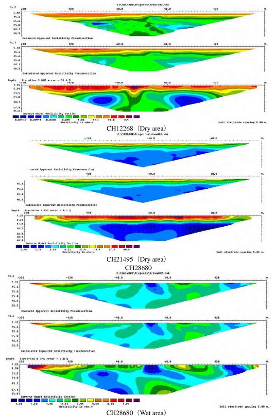
Figure 4.2.15 Map of soil resistivity (Longitudinal)
