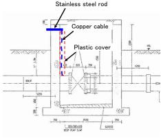
Figure 4.2.30 Terminal for monitoring of CP
