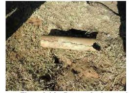
Figure 9.4.2 Damaged asbestos pipe
