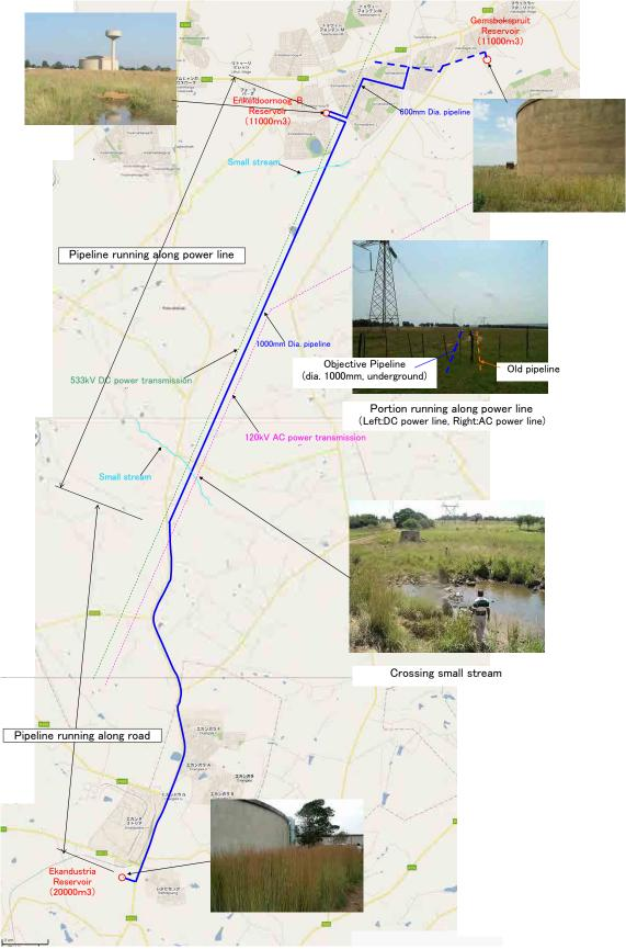
Figure 4.2.2 Route of the pipeline
