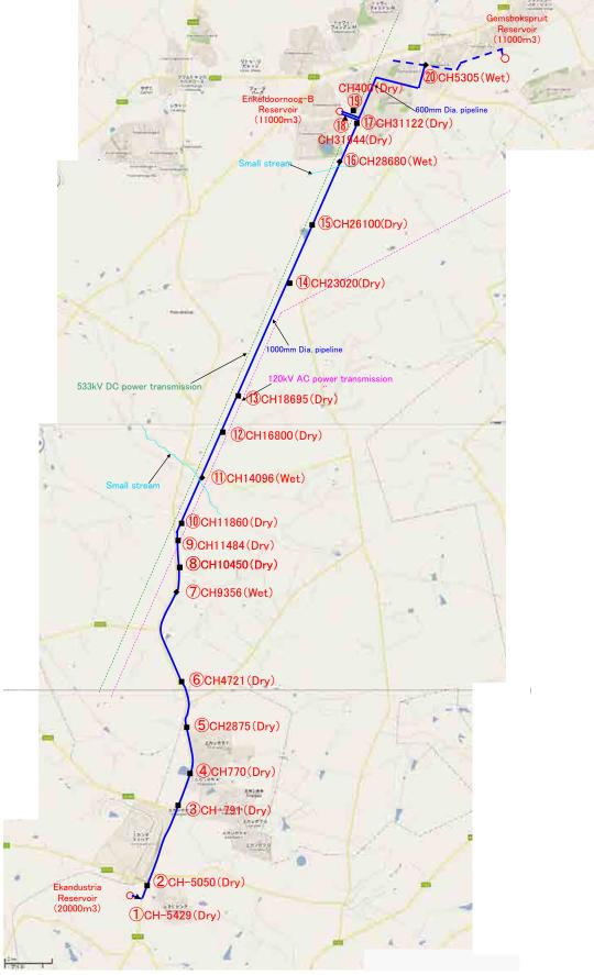
Figure 4.2.11 Measuring points for pipe to soil potential and soil resistivity (20 points)
