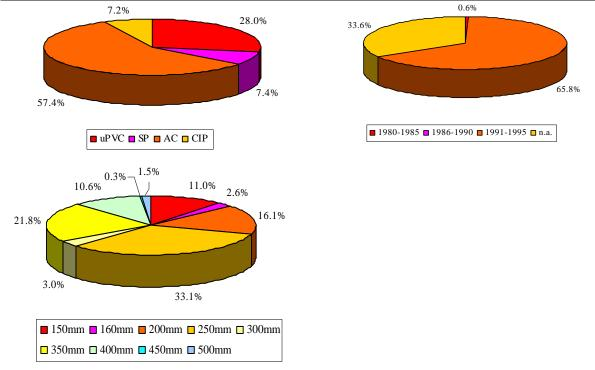
Figure 9.7.4 Status-Quo of Bulk Water Pipelines in Sekhukhune DM
