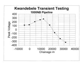
Figure 4.2.28 Change of potential at load changing of DC transmission line(From survey in 1999)
