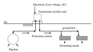
Figure 4.2.25 Impressed current cathodic protection
