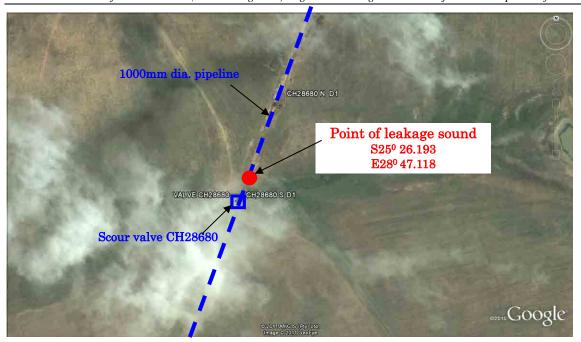
Figure 4.2.19 Point of leakage sound detected
