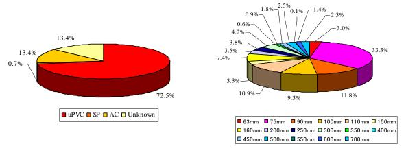
Figure 9.7.5 Status-Quo of Reticulation Water Pipelines in Kungwini DM
