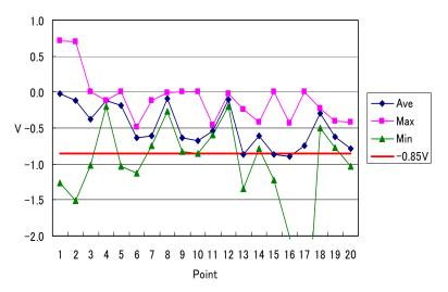
Figure 4.2.7 Measurement of PS potential (Graph)
