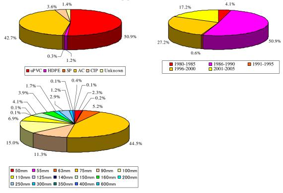
Figure 9.7.7 Status-Quo of Reticulation Water Pipelines in Sekhukhune DM
