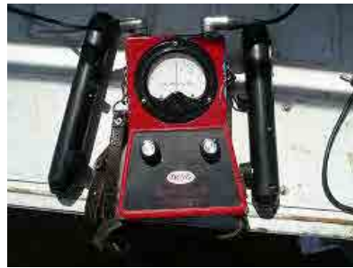
DCVG survey (Equipment)
