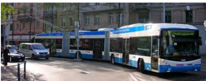
Figure 6.4.38 The multicar set of a bi-articulated bus with electric propulsion resembles an LRT system
