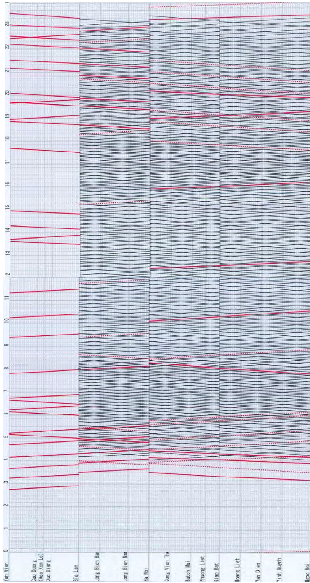
Fig. 3-6: Train diagram for simultaneous opening of Phase 1 + 2a in 2020 (Red line: hauling trains for locomotives; Black lines: electric trains of urban railways)
