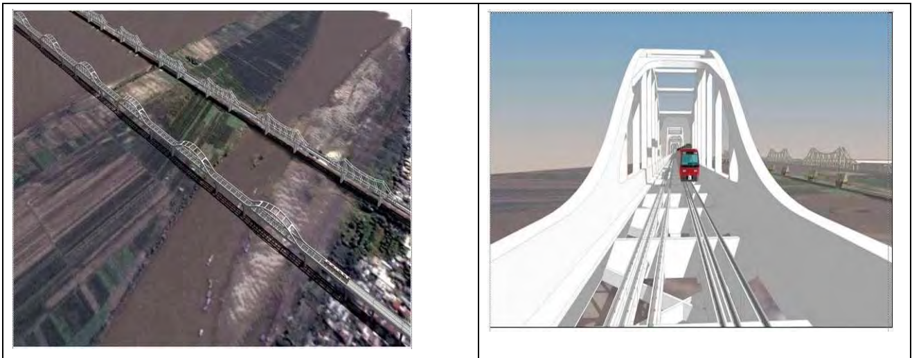
Figure 3.3 Perspective of new Long Bien, balanced solid rib arch
