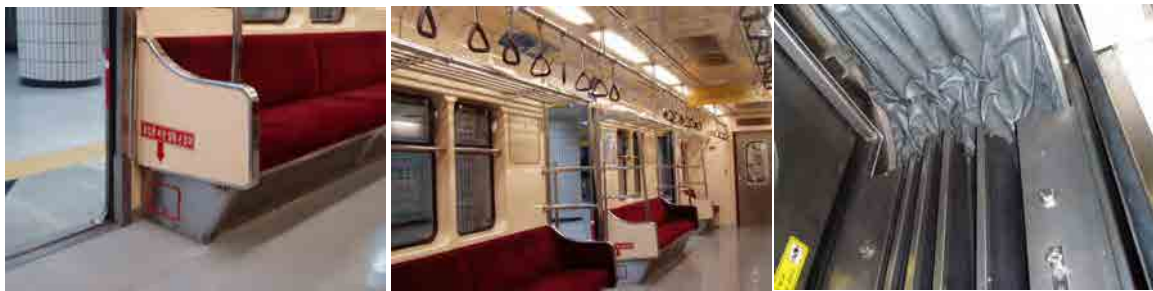
Figure 2-10 Combustible Material in the Rolling Stock of Dague Metro (Polyester, Urethane Foam, FRP, etc.)
