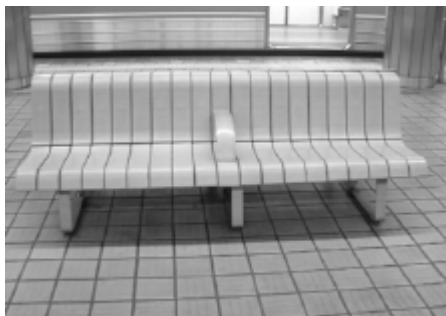
Figure 2-1 Use of non-combustible material for the chair in the station
