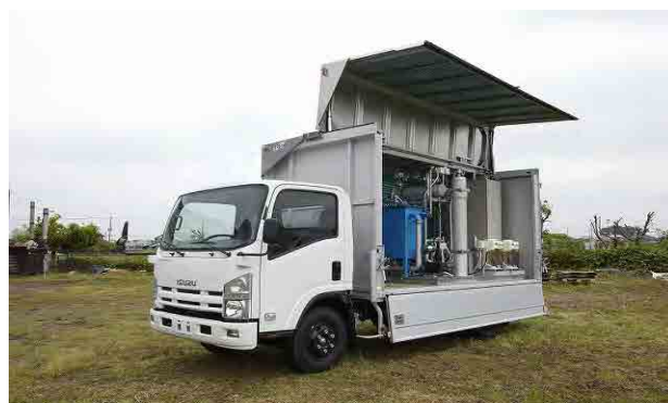
Figure 5-5 Mobile ceramic membrane filtration equipment (M-CMF) (50 m 3 /day)
