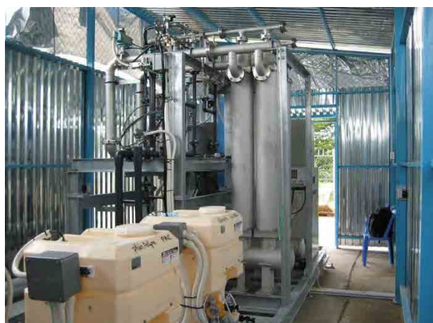
Figure 5-4 Small scale ceramic membrane water treatment system (240 m 3 /day)
