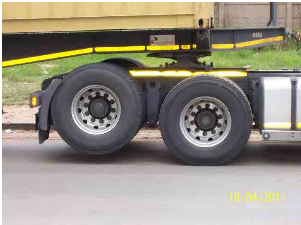
Photograph 6-5: Truck Tractor with Lifiable "Tag" Axle
