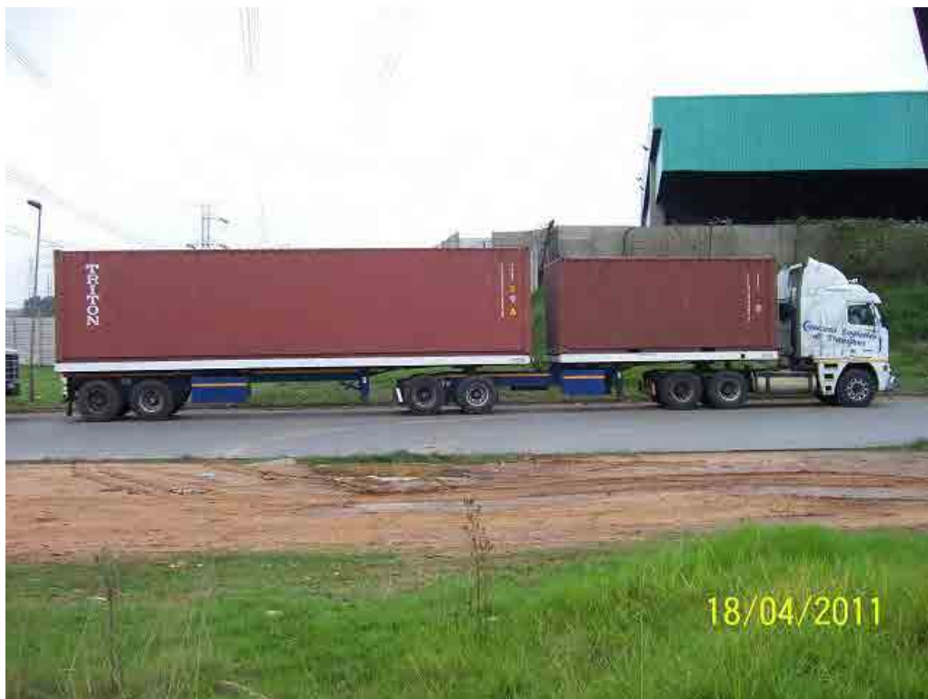
Photograph 6-12: Flat Deck Interlink with 1 × 6 m and 1 × 12 m High-cube Containers
