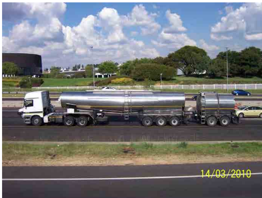
Photograph 6-1: 56-tonne Semi-trailer and “Pup” Combination, with 385/65R22.5 Tyres on the Trailers
