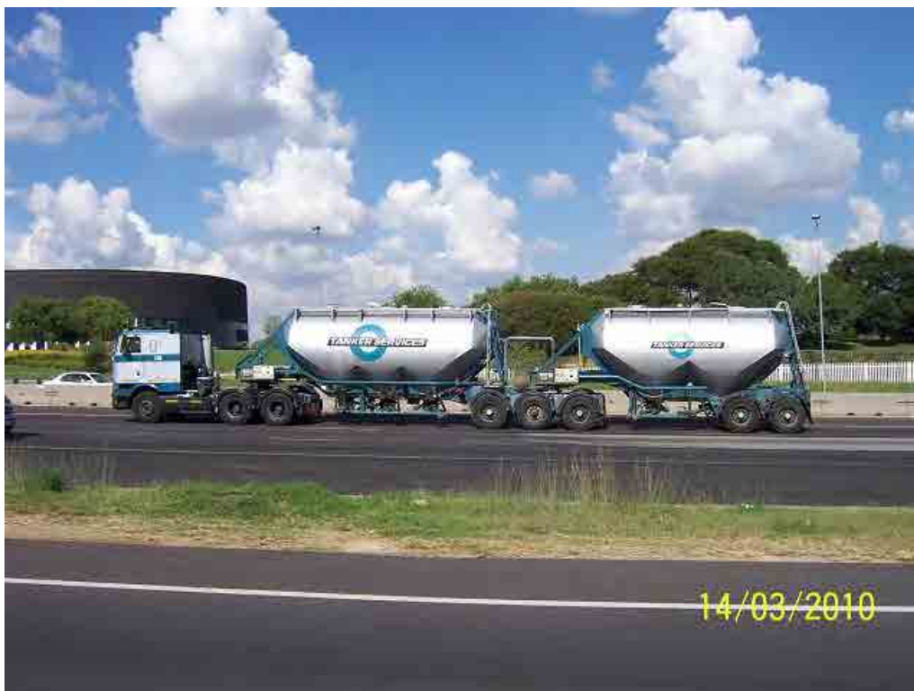
Photograph 6-10: Bulk Cement Interlink with Super-single Tyres
