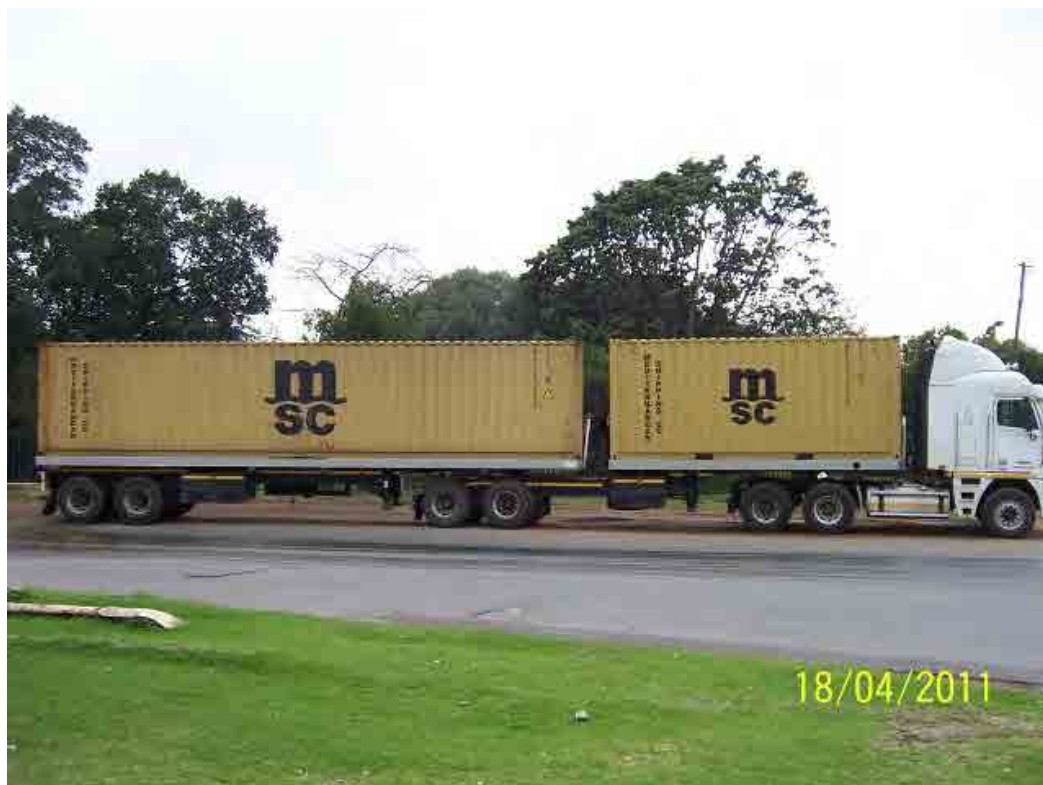
Photograph 6-13: Flat Deck Interlink with 1 × 6 m and 1 × 12 m Containers
