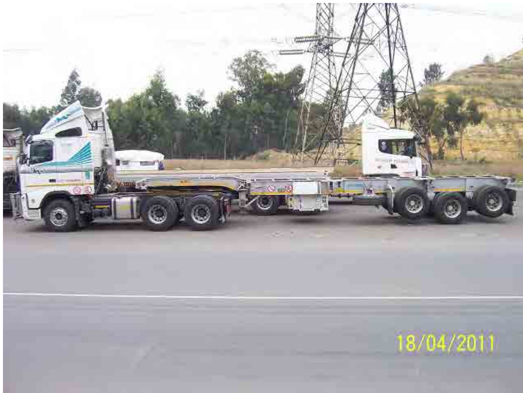
Photograph 6-2: Semi-trailer with Two Lifiable Axles
