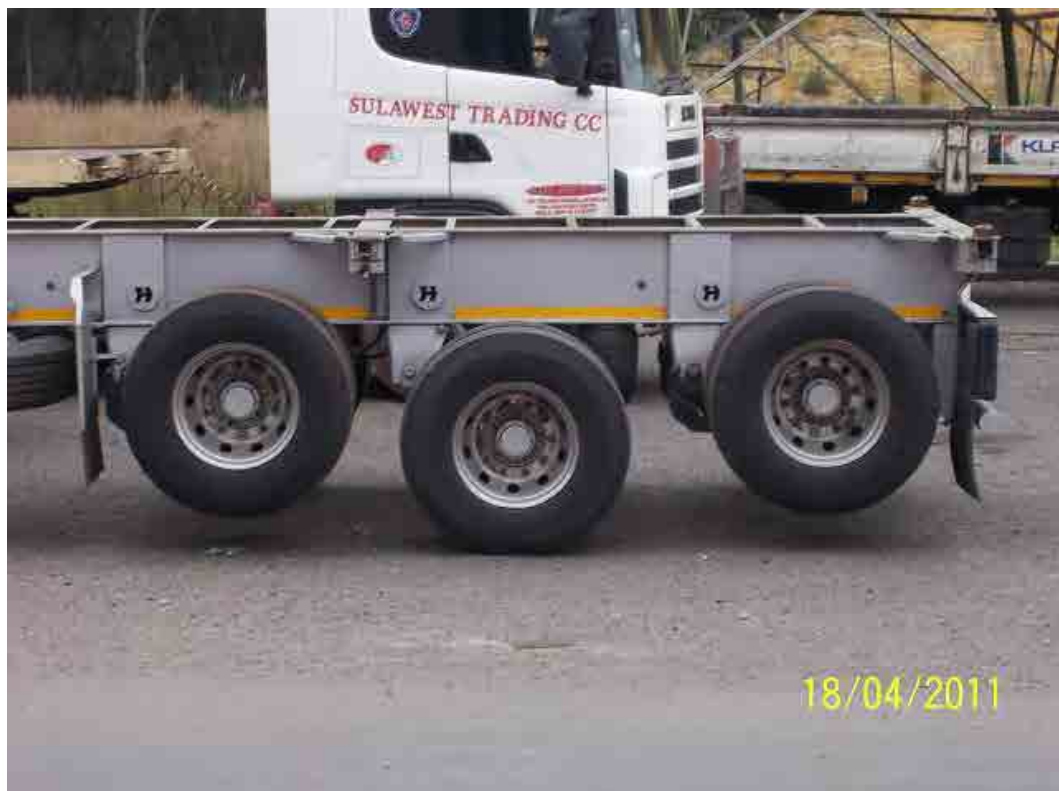
Photograph 6-3: Two Lifiable Axles on a Semi-trailer
