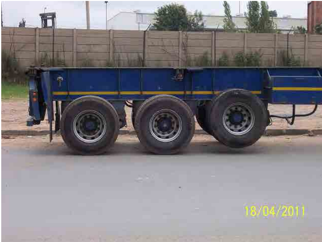
Photograph 6-4: Semi-trailer with One Lifiable Axle
