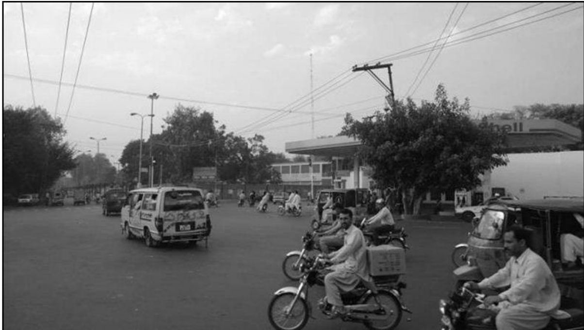
Figure 8.5.3 Poor Gyratory System Design without Traffic Channelization
