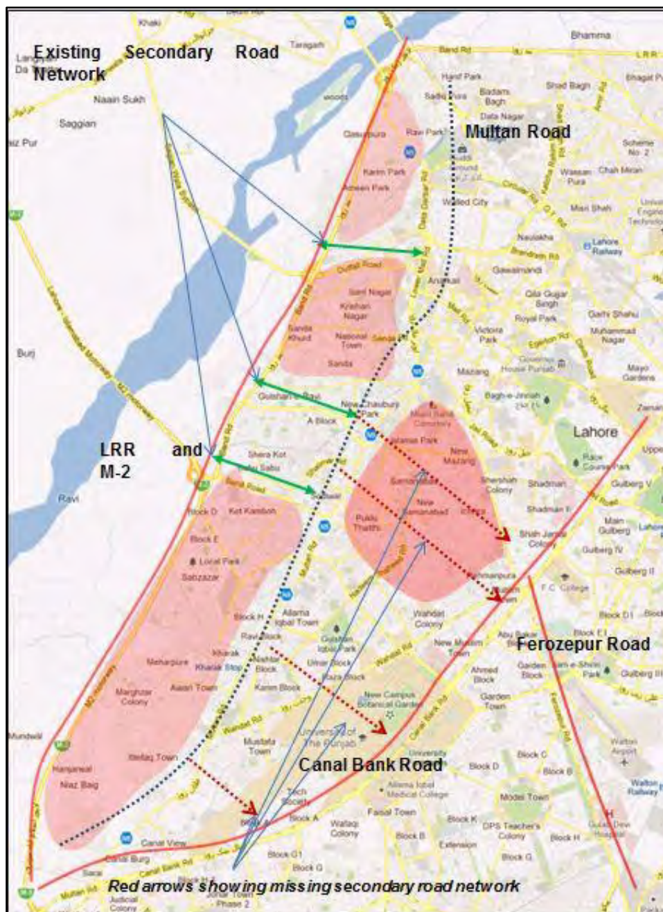
Figure 8.6.2 Samanabad Area Lack of Internal Secondary Roads and External Linkages
