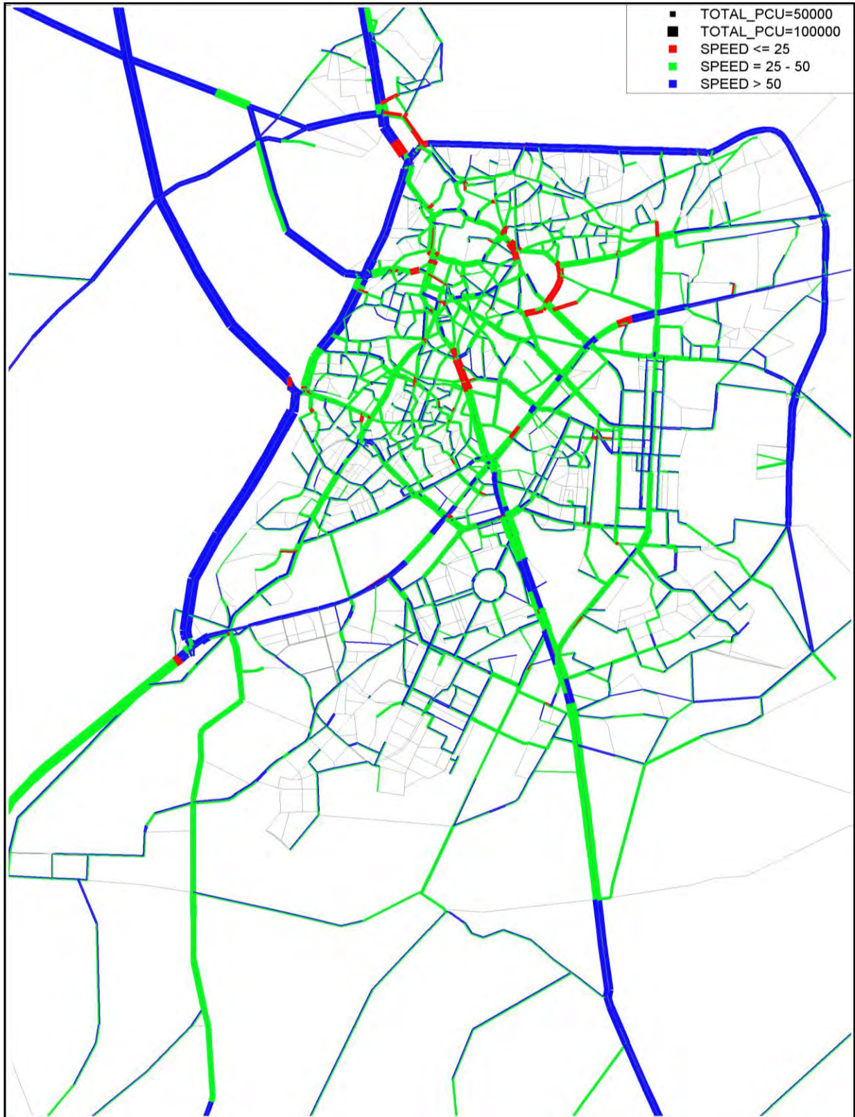
Figure 7.2.2 Current (2010) Road Network Performance
