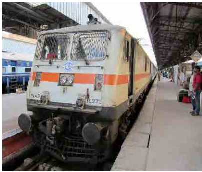
Figure 3-2 Express in Operation with Window Broken by Flying Stones
