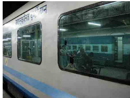
Figure 3-2 Express in Operation with Window Broken by Flying Stones
