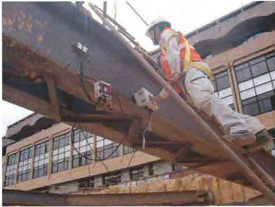
Installation of Strain Gauge for Strut Axial Force at Cricket Stadium Station
