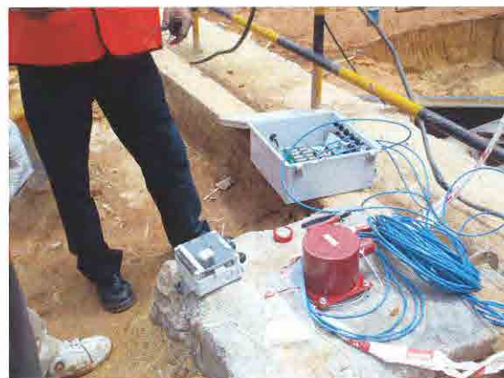
Installation of Inclinometer and OSV Display Equipment at Cricket Stadium Station
