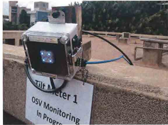
Inclinometer on Secant Pile and Lighting Conditions (Blue) at Cricket Stadium Station
