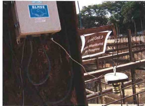
OSV Display (Blue & Yellow) for Ground Anchor Axial Force at Central College Station
