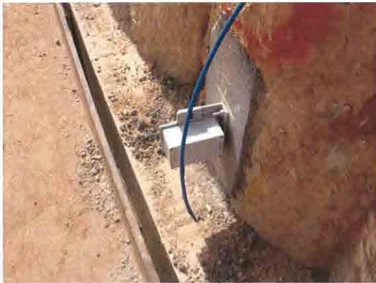
Inclinometer on Secant Pile and Lighting Conditions (Blue) at Cricket Stadium Station
