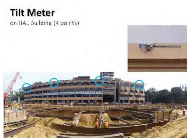
(a) Locations (blue circles) of tilt meters
