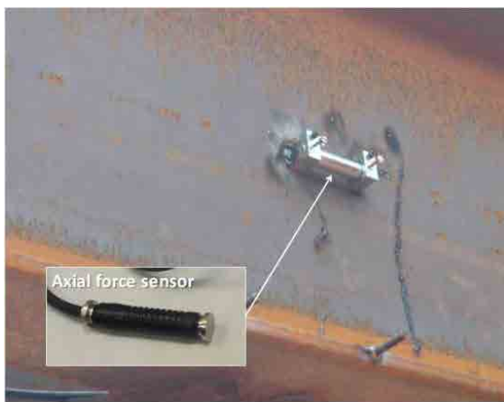
(b) Axial force sensor welded to a beam
