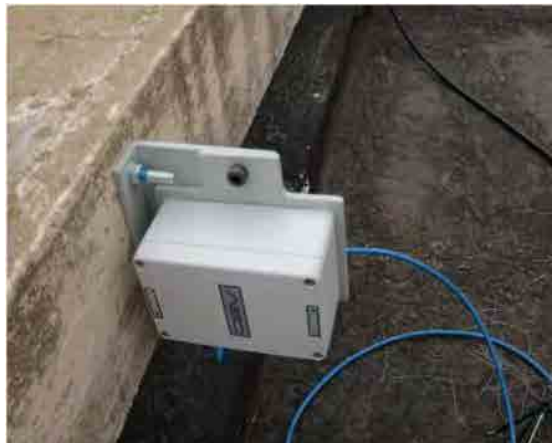
(b) Tilt meter supplied by Encardio-Rite (India)
