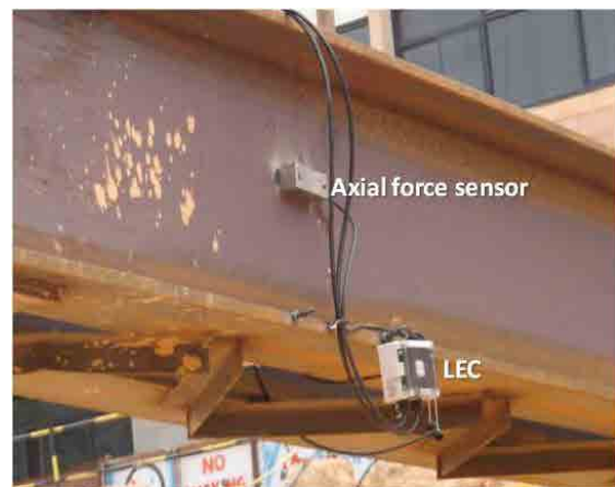
(c) Axial force sensor connected to LEC
