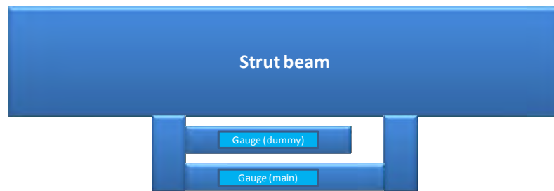
Figure 3.18 Fundamental structure of an axial force sensor with automatic temperature compensation
