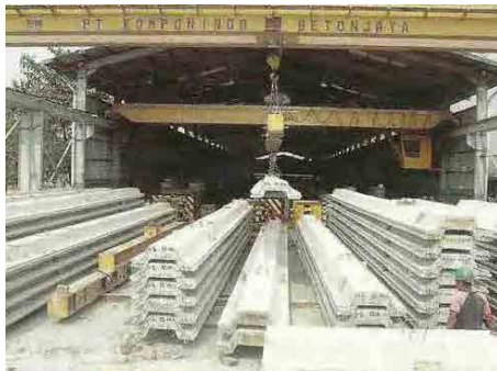
Photo-5: Precast PC Sheet Piles
