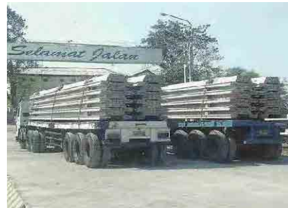
Photo-6: Transport of PC Sheet Piles
