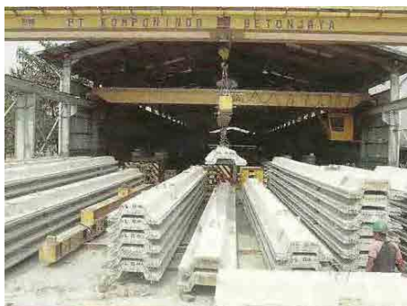
Photo-5: Precast PC Sheet Piles
