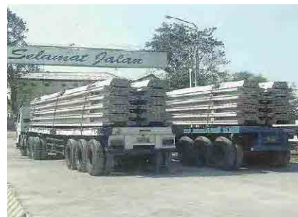
Photo-6: Transport of PC Sheet Piles
