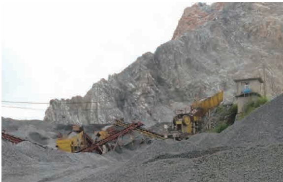
Figure 3.2.3-15 Quarry using impact breaker
