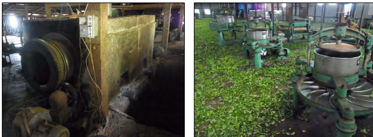
Figure 6-24 Cooking Oven (left) and Kneaders (Phongsaly province)
