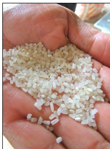
Figure 5-3 Low Head Rice Ratio under Current Milling Technology is a Bottleneck for Exportation (A Rice Mill in Vientiane Province)
