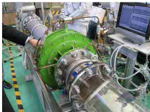
Ring turbine (Tsuyama Municipal Water Department unit)
