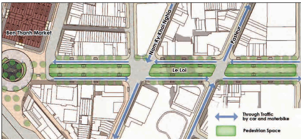
Figure 4.30 Ground Level Plan of Le Loi Street (based on Urban Planning of Ho Chi Minh City)
