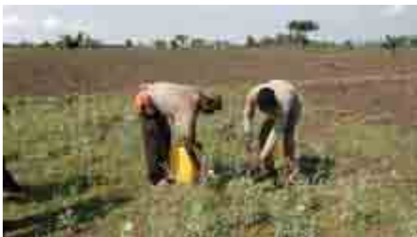
Oyne Umbure BH-3 (Watering of electrodes to reduce contact resistance )
