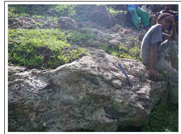
Fig.9: Boundary between welded tuff and pumice tuff. Boundary is unclear; which is considered that those formations might be single cooling unit.
