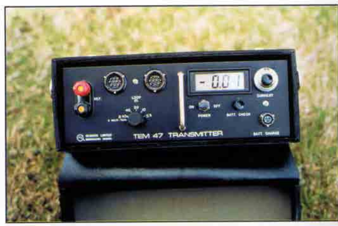
TEM47 Transmitter (Frequency of 75Hz)
