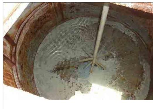
Inside of mixing tank. Some residue of chemicals is seen at the bottom.
