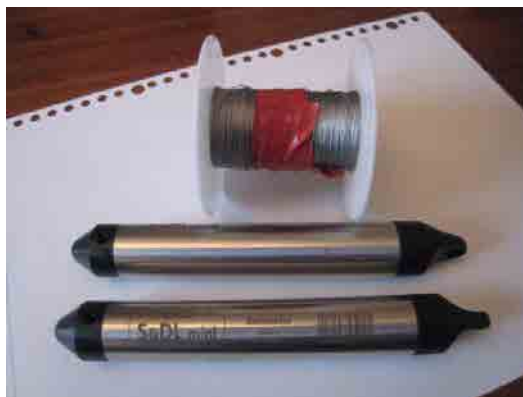
Figure 5.37: WLR employed (OYO S&DL mini) and wire
