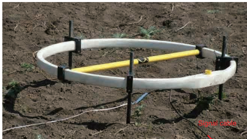
Protom Receiver Coil (Low Frequency) Rx
