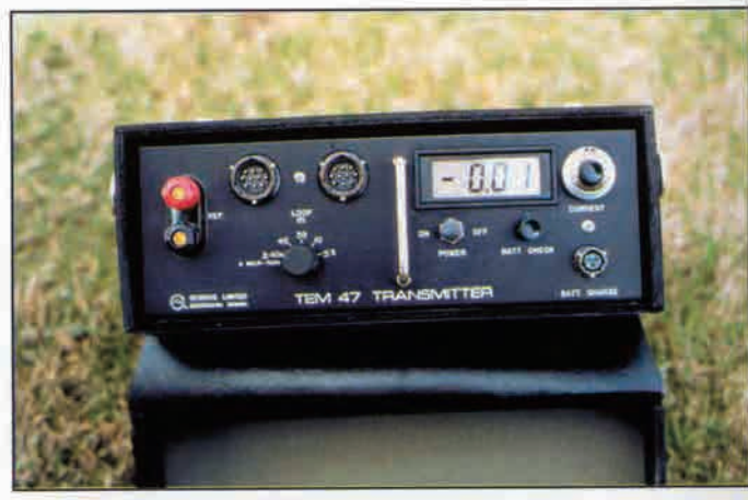
TEM47 Transmitter (Frequency of 75Hz)
